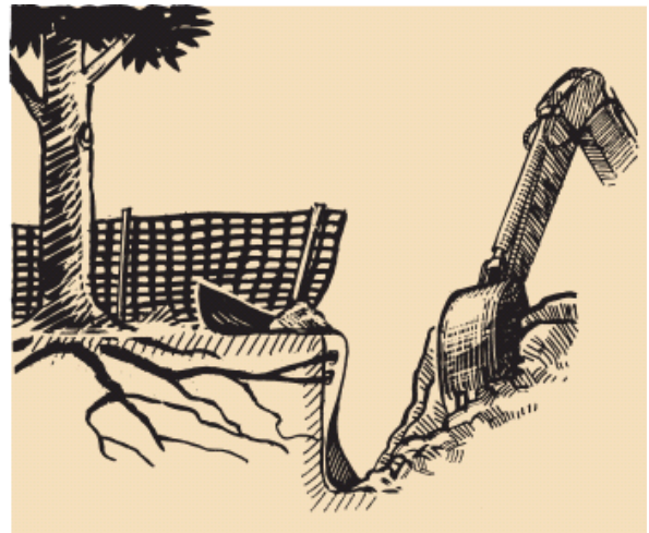
Figure 27. After roots are exposed and cleanly cut, the soil around them should be watered and covered with black plastic during hot periods. Large equipment can be used for mass grading after tree roots have been protected.
