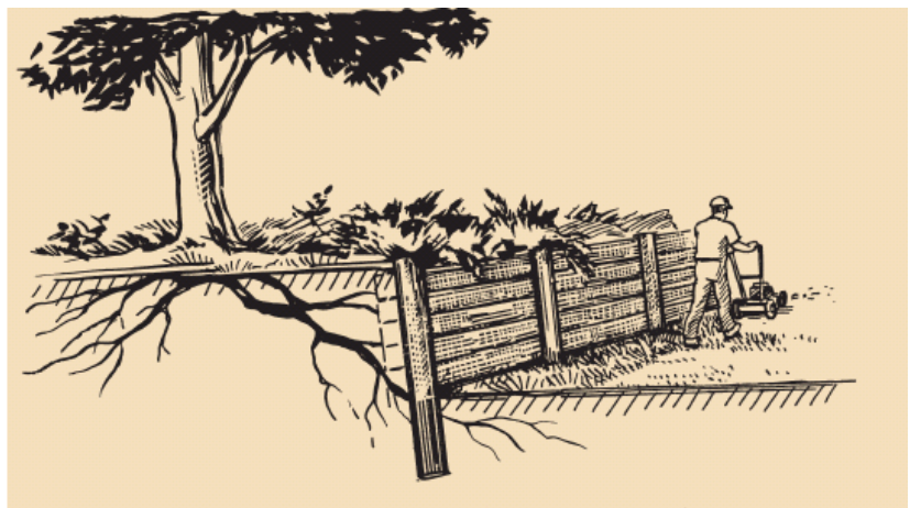
Figure 14. Crib walls can be used to limit the length of manufactured slopes, providing more room for trees and development.
