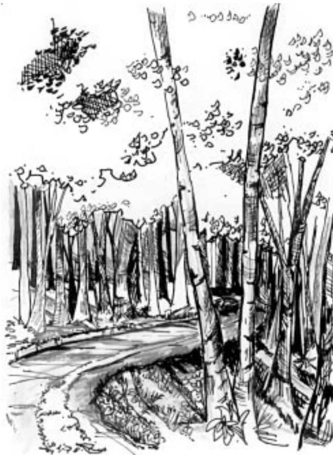
Figure 3. This access road follows the natural horizontal contour of the land and is well vegetated on both sides, thus minimizing water run-off and soil erosion.
